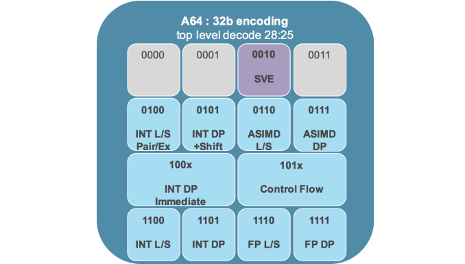
(a) A64 top-level encoding structure, with SVE occupying a single 28-bit region.
